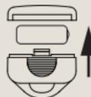
Replace battery and slide cover back into position
