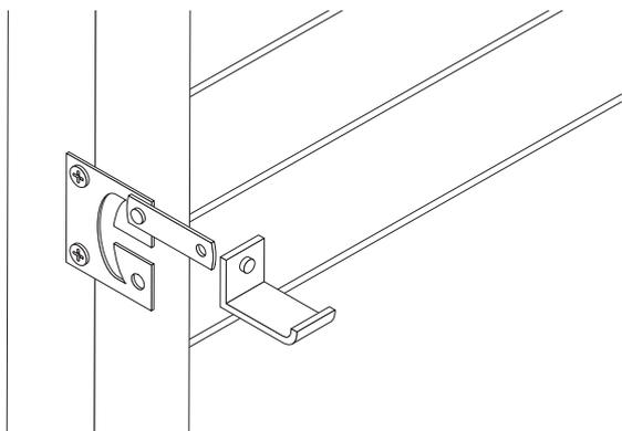
Attach the round bottom rail stop to the bottom rail with the bottom edge of the stop level with the bottom edge of the bottom rail.
