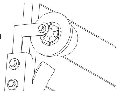
The extruded guide head stops should be attached as shown using self drilling screws to the cavity section of the guide.
