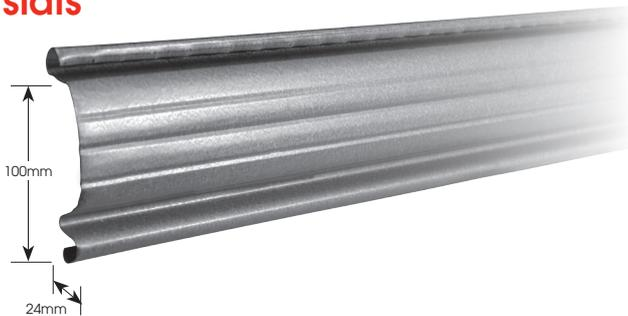
High tensile G550 continuous roll formed, interlocking, coated Galvabond® steel slats. Nominal effective pitch of 100mm with 3 small ribs. Zincalume® coating of not less than 150g/m<sup>2</sup>. Moulded nylon clips fitted to end of alternate slats by means of three nylon rivets.
