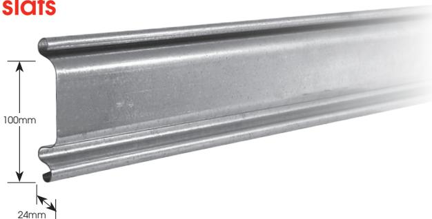
1.0mm, continuous roll formed, interlocking, coated galvanised steel slats. Nominal effective pitch of 100mm. Zinc coating of not less than 275g/m<sup>2</sup>.
