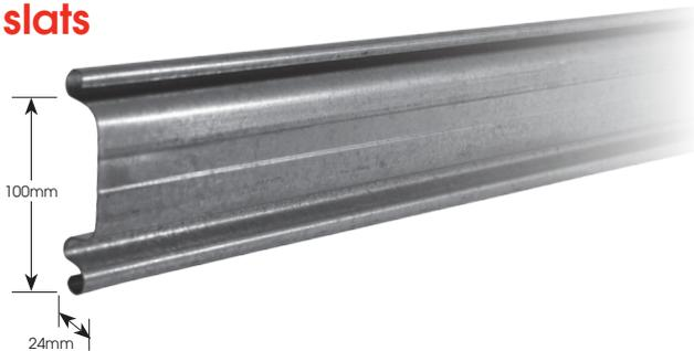
0.6mm, continuous roll formed, interlocking, coated galvanised steel slats. Nominal effective pitch of 100mm. Zinc coating of not less than 275g/m<sup>2</sup>.
