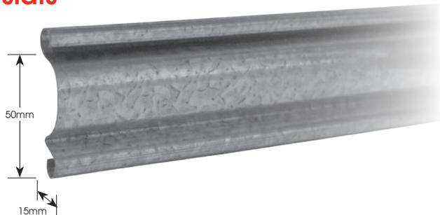
0.8mm, continuous roll formed, interlocking, coated galvanised steel slats. Nominal effective pitch of 50mm. Zinc coating of not less than 275g/m<sup>2</sup>. The curtain is fitted with moulded nylon clips to the ends of alternate slats by two nylon rivets.
