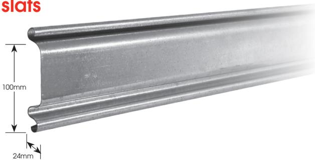
1.0mm, continuous roll formed, interlocking, coated galvanised steel slats. Nominal effective pitch of 100mm. Zinc coating of not less than 275g/m<sup>2</sup>.
