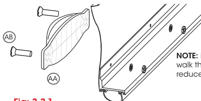
**NOTE:** if handle is fitted the walk through height will be reduced by 80mm.
