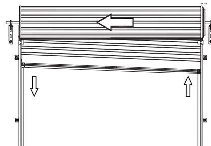
If the door rolls up crooked with the **LEFT HAND SIDE** higher than the left proceed as follows:
