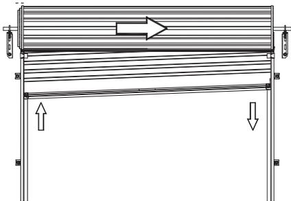
If the door rolls up crooked with the **RIGHT HAND SIDE** higher than the left proceed as follows:
