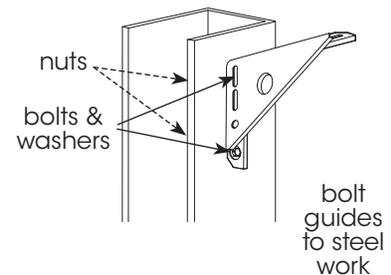
**WARNING!** Masonry blockwork should be properly filled and reinforced if brackets are to be mounted directly to blockwork with masonry anchors. Where the blockwork is not solidly filled but structurally sound, long bolts should be passed through the blockwork using suitable steel plates under bolt heads. Special consideration should be given to brick type and construction of wall, to ensure satisfactory fixing.
