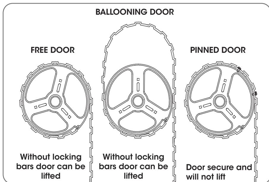
**WARNING!** It is the installers responsibility to choose a fastener length that will adequately secure the curtain to the drum.
