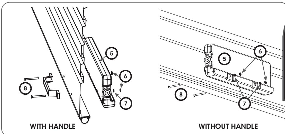
**WARNING!** To reduce the risk of damage to persons or property, be sure to cut off any excess thread of the screw that protrudes the weight bottle and file any burrs.
