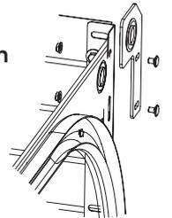
**NOTE:** The small angle jamb brackets and the top angle bracket, provide adjustable slots to move the track out from the wall. Take note of Fig 3.1.2 for measurements.
