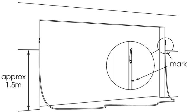
2. Mark equal overlap at each side based on panel width.
