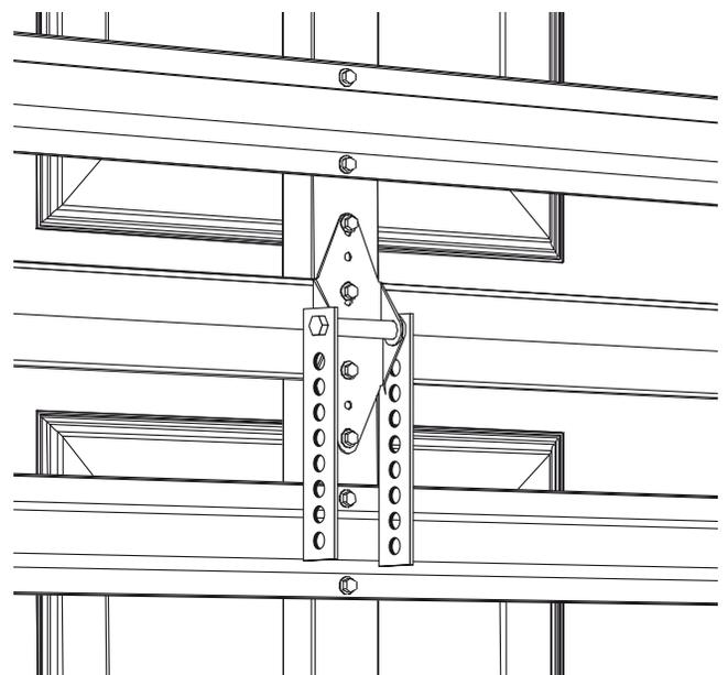
Now stand the aluminium brace in position, ensure it is plumb in line with the hinges, adjust the 'U' bolt so that it fits comfortably in the lintel bracket and the brace has 5-8mm clearance from the panel reinforcing, Figure 2.11.2.
