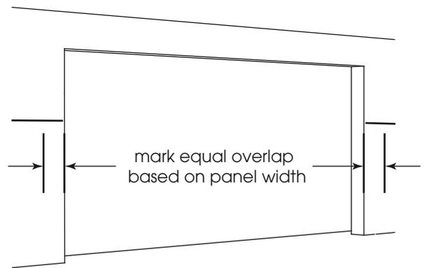
3. Mark the track position 45mm from the previously marked panel width.
