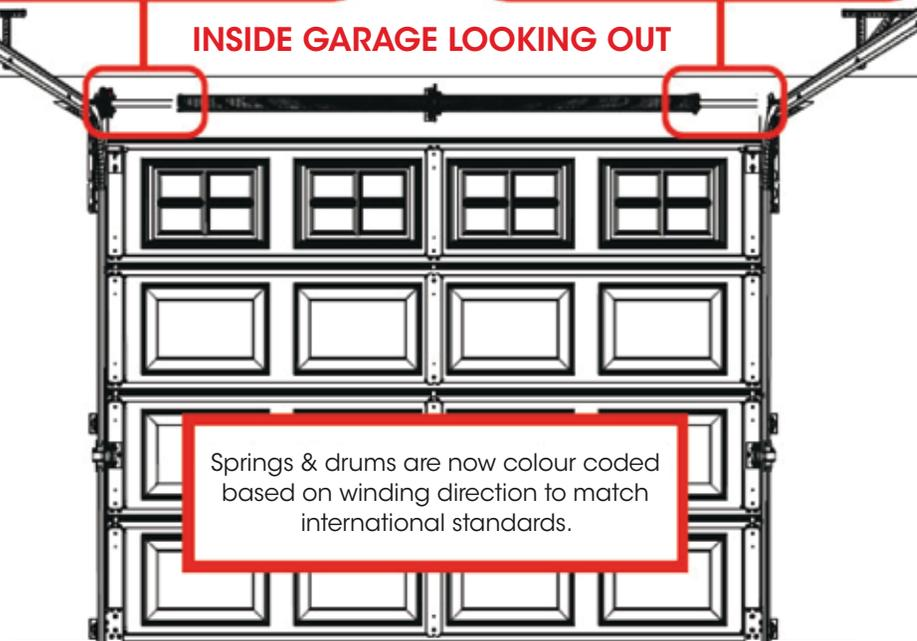
Springs & drums are now colour coded based on winding direction to match international standards.
