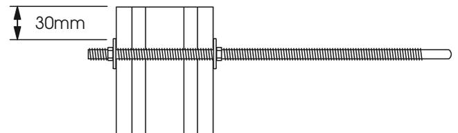
Stand the aluminium brace to one side, fit items O, P and M to the hinges as shown in Figure 2.11.7 directly under the lintel bracket to every hinge.
