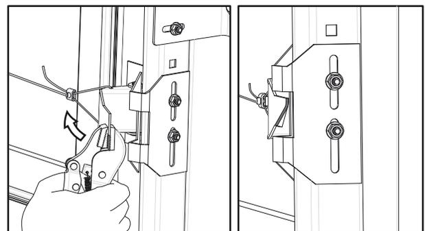
Figure 3.1.6 modification to lock when tracklocks are fitted (not supplied)
