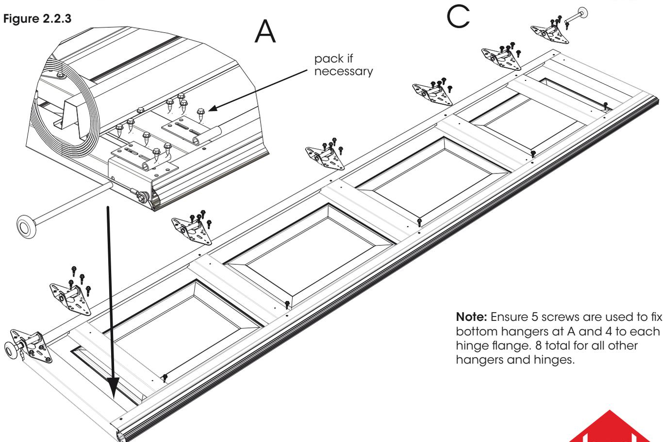
**Note:** Ensure 5 screws are used to fix bottom hangers at A and 4 to each hinge flange. 8 total for all other hangers and hinges.
