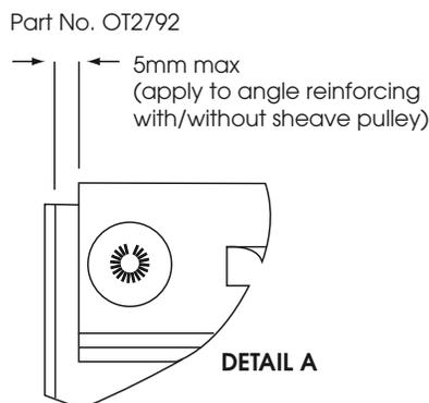
1. Mount sheave pulley and angle reinforcing bracket sub-assembly as per instructions for Bracket (OT2791).
