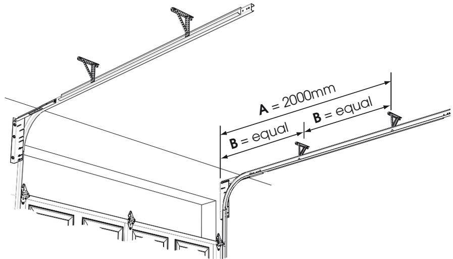
Figure 2.5.4 installing the safety stop
