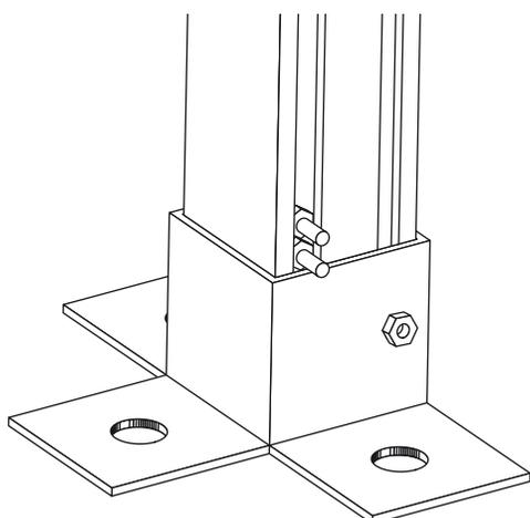
Assemble the "U" bolt as shown and fit over the top of the aluminium brace Figure 2.7.5.
