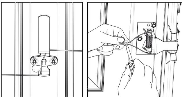
Figure 3.1.5 bending lock strike
