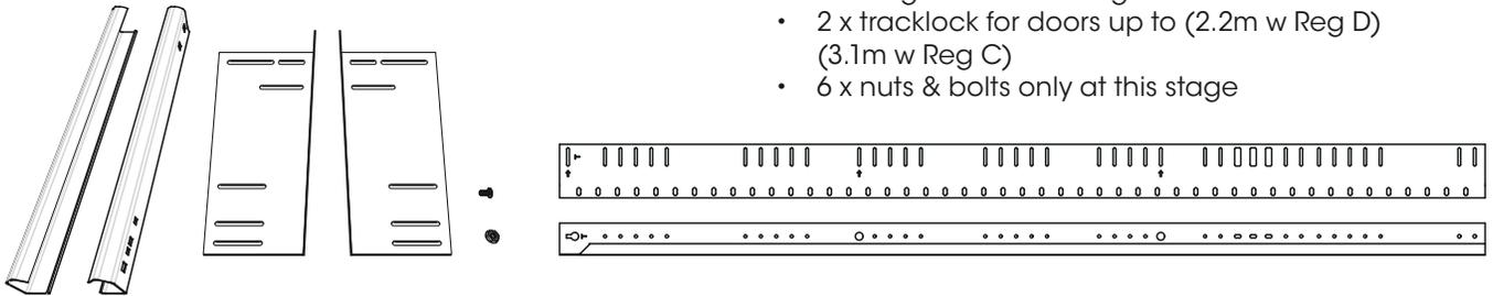
Note the 'T' mark on the lower track bracket and tracklock to indicate top. Only the bottom must be cut to suit door height.
