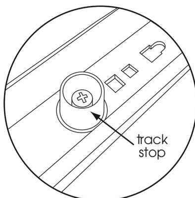
Safety stops must always be fitted at the end of each horizontal track.
