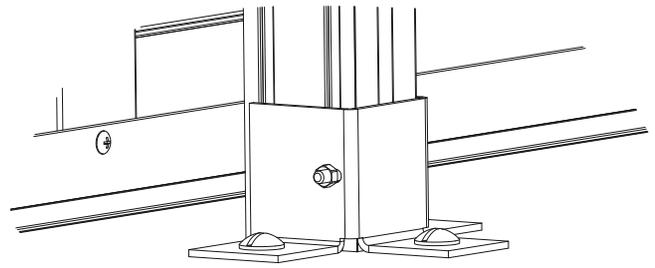
Stand the brace in position make sure it is hooked in place at the lintel and insert three dome head (S) fixing screws into the three floor anchors.
