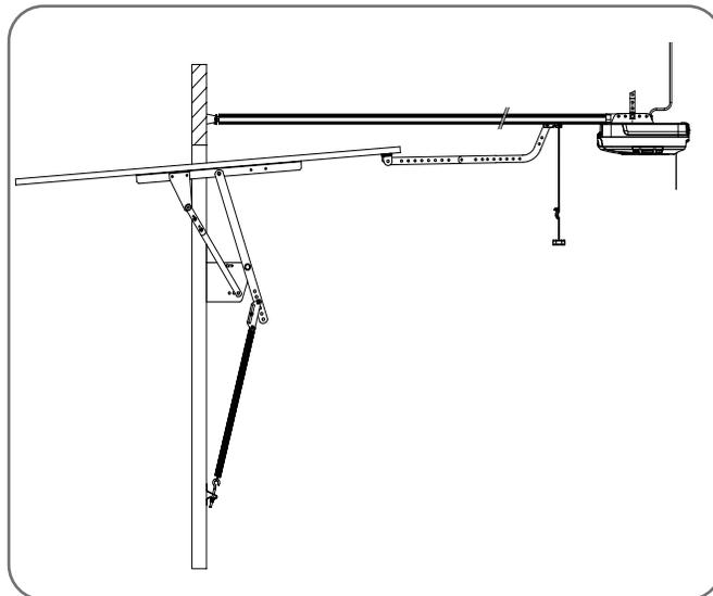
Prior to limit set up, the opener can be set to J-Type Tilt Profile. This process allows the opener to pre-set to J-Type settings where the limit is not greater than 1500mm.
