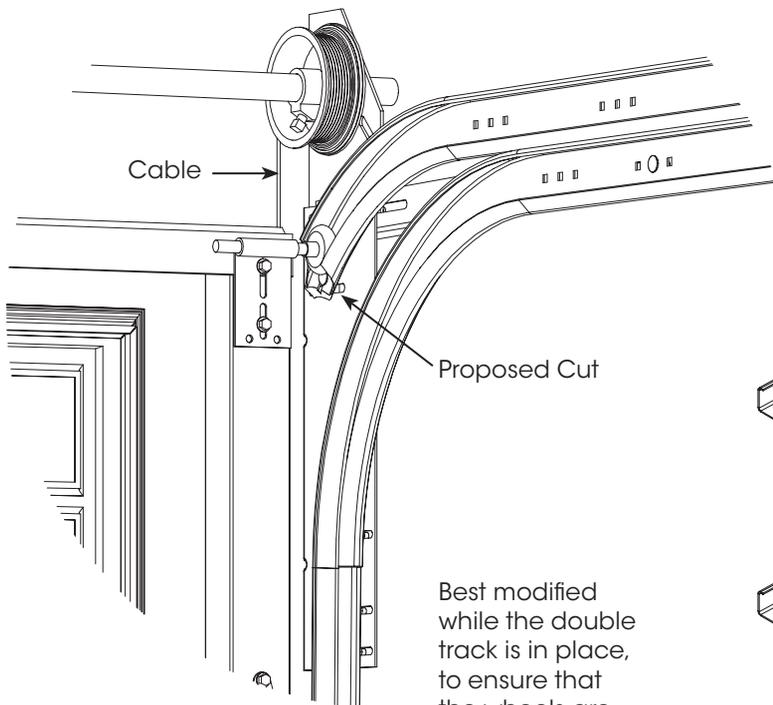
The top track curve needs to be 'trimmed' so as not to interfere with the cable during operation but still firmly retains the trolley wheel. A suitable cut can be shown below.
