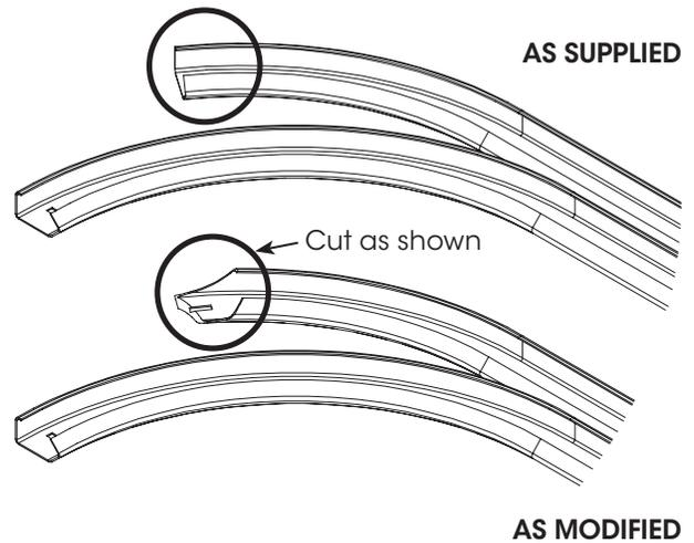
Best modified while the double track is in place, to ensure that the wheels are retained.
