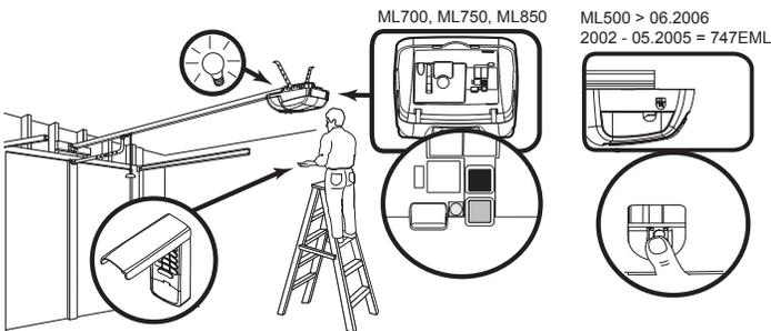
1. Press and release the learn button on motor unit. The learn indicator light will glow steadily for 30 seconds.
