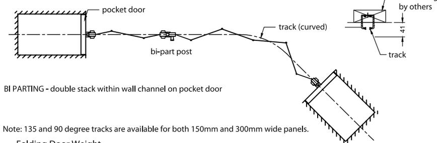
Note: 135 and 90 degree tracks are available for both 150mm and 300mm wide panels.
