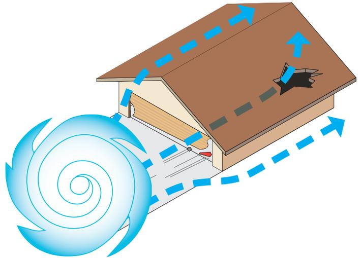
If you live in high wind and cyclonic areas, it's necessary to engineer your garage door a little differently to ensure it withstands the particular stresses it may be subject to and minimise the potential damage to your home.
